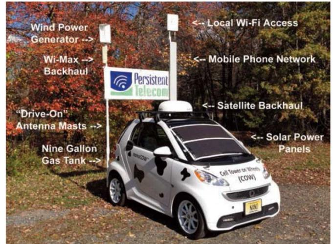
The nanoCOW™ design team learned an important lesson during Superstorm Sandy - establishing an emergency cell site was easy when compared to the effort needed to re-fuel the generators to keep the sites powered up.
